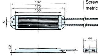
Braking resistor unit (separately-installed type)
