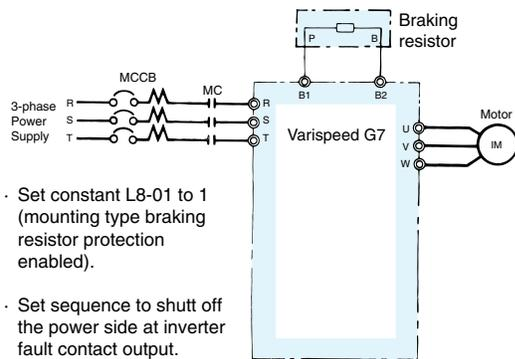
**Connections for braking resistors**
