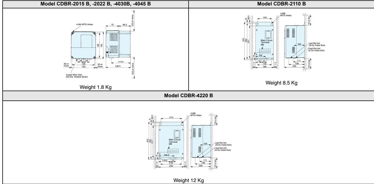
Braking resistor unit (inverter-mounted type)
