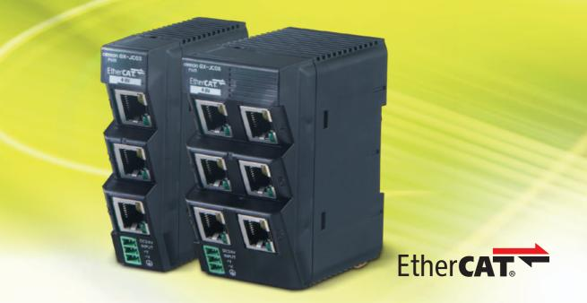
Daisy chaining, star wiring, and tree connections can be made in one network. Efficiency in assembling and wirings will be improved, shortening the time required to start the system operation.
