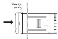
3. Insert the fixture into the grooves on the left and right sides of the rear case and push until it reaches the panel and is fixed in place.
