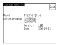
The system program's version information will be displayed as described below. Press the Quit touch switch to exit the Version Display screen and return to the Expansion Mode screen.
